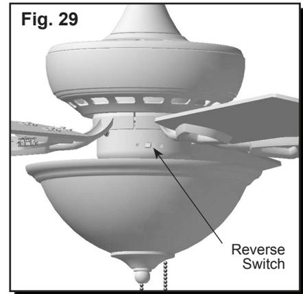
30. **In warmer weather**, push the reverse switch left, which will result in downward airflow creating a wind chill effect (Fig. 30).
